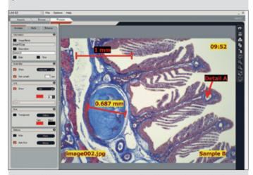
Process: After image capture you can easily add annotations and basic measurements to the images. A gallery of images stores all the calibration and camera data for fast reference.
