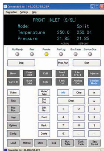
A “virtual keyboard” allows you to control the instrument when you only use the data handling solution.
