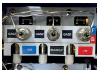
New Electronic Pneumatic Control (EPC) module for the 7820A GC.
