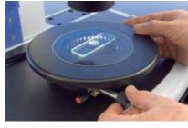
Equipped with a gliding stage, salient positions on the specimen can be brought into position easily, without jostling the sample.
