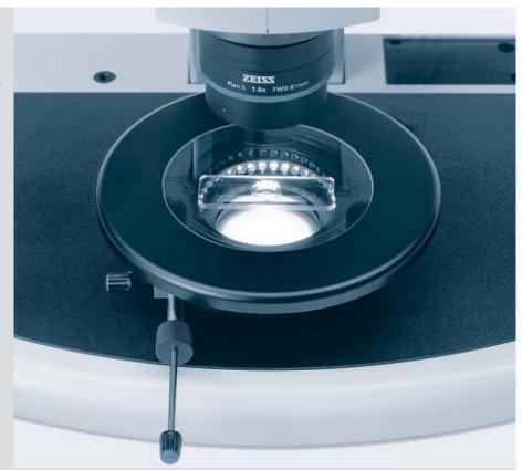
VisiLED transillumination BF, d = 84 mm Retrofitted into the Stand base 450 to Profile S or the Stage carrier S for simple transmitted-light brightfield applications.
