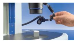
Extremely precise alignment of the illuminator is a must in order to achieve good 3D contrast in oblique reflected-light. Special clamps, illuminator carriers and articulated arms are available to ensure that the fixing is exact. Focusing attachments help to concentrate the light on the object field.
