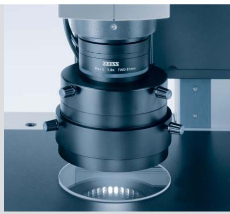
In order to combine brightfield and darkfield in reflected-light, the VisiLED ring light S 40-10 DF is mounted onto the brightfield ring light using a special adapter.
