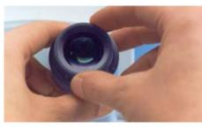
All eyepieces can be focused and, therefore, allow individual adjustment for both eyes..
