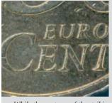
While the contours of the striking on this cent coin are highlighted in particular in darkfield, in mixedlight it is primarily the irregularities of the surface that are revealed more clearly.
