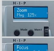
The wheel responds dynamically to the movement of the thumb: slowly and sensitively with small movements and more quickly with larger movements.
