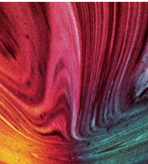
Section of plastic component, polarization
