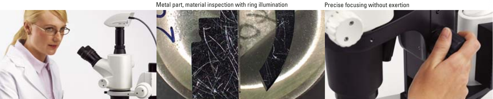
Metal part, material inspection with ring illumination
