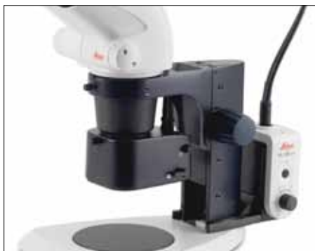
Coaxial illumination for flat reflective objects such as polished metal components, wafers, chips, or layered surfaces.
