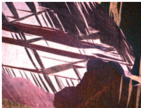
Tin with deformation twins, 1:100
