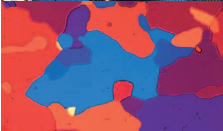
Aluminum, Barker etching, polarization
