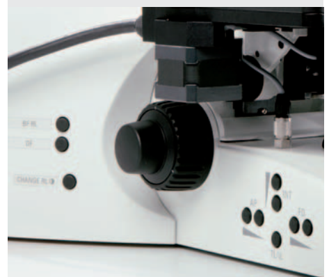
Configure specific illumination and diaphragm settings with the buttons on the left front side.
