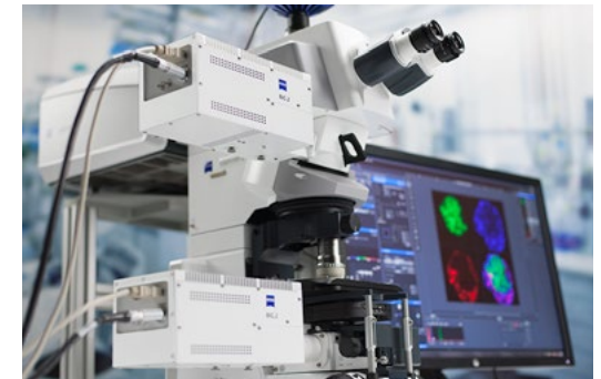
BiG.2 works perfectly as a non-descanned detector, also providing a highly sensitive direct coupled detector for FLIM.
