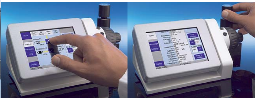
The TFT display on the stand or in the docking station provides a transparent menu guide for control and configuration.
